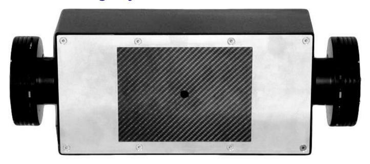
We have developed an inexpensive replacement for the old Polaroid Laue camera consisting of a dual-CCD camera with real-time read-out. Large aperture lenses are used to image the scintillator onto the CCDs, which also have micro-lenses over each pixel. This camera is similar to the old Polaroid Laue camera, in being simple, efficient and low cost, but the image is available immediately for the determination of crystal orientation.
