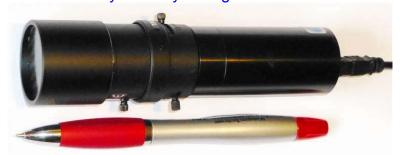
Our <u>mini i-Cam camera</u> could be used to maximise the beam and position the sample, otherwise use the Laue camera itself to image transmission through the collimator.
