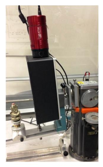
**Left photo:** The Huber IP camera is the circular disk mounted on a blue support on a guide rail. The collimator is locked and the beam shutter opened with the two black knobbed levers on the double-metal plates that form the <u>Huber-800</u> alignment mechanism, which is mounted on a 1960's Philips X-ray generator. The screw at the top, and two at the bottom, adjust the height and tilt of the collimator.
