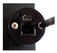
The CCD unit backplate can be removed by unscrewing the two screws, and then the black metal shell can be simply pulled off to reveal the motherboard, which is held by two hexagonal metal columns. You can then check the USB socket.
