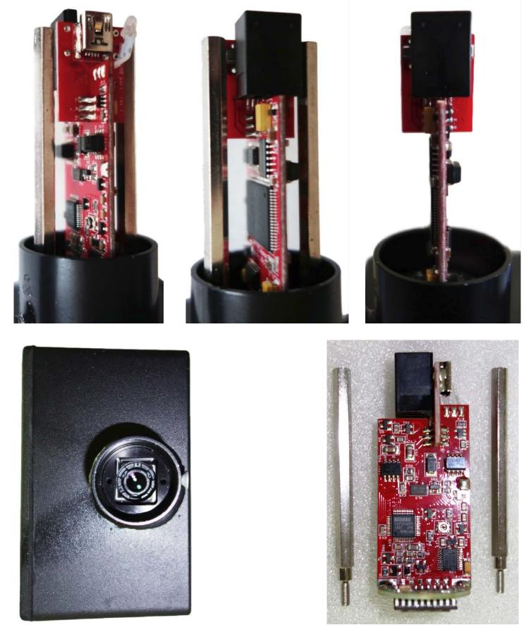
The left photo shows the base of the lodestar CCD unit, still held by its locking screw. The right photo shows the lodestar motherboard with the two hexagonal pillars that screw into the base to hold it. The CCD chip is at the bottom of the motherboard, and must be re-located in the rectangular hole in the base (left) through which the rear of the lens can be seen.
