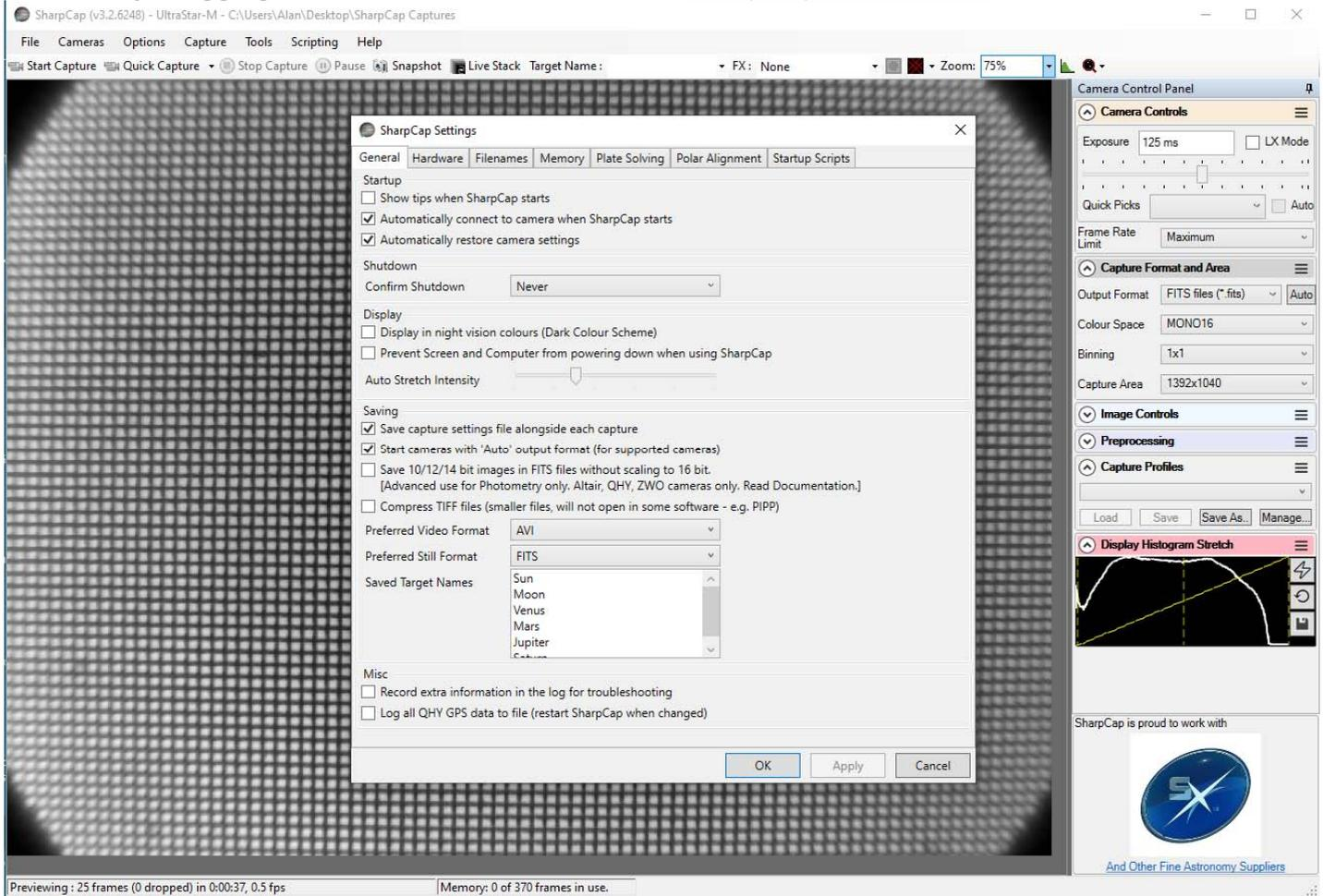
In the Camera Controls you can **set the Exposure** (toggle LX mode for long exposures), and for some cameras the gain (higher gains increase noise) and sensor temperature. In the Capture Format, select TIFF or FITS and Mono16. Select **Sum Odd & Even rows and expand**. To speed up readout, select a reduced Capture Area, and drag the rectangle to the Region of Interest, and Zoom to magnify. You can also drag the vertical line in the Display Histogram to stretch the intensity display.
