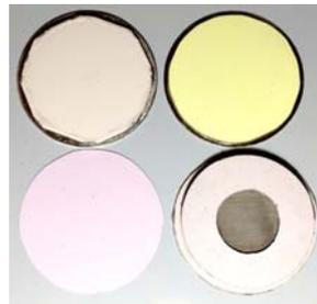
**Scintillators:** 20 $\mu$ m GadOx, 450 $\mu$ m LiF, OG2 x-ray, and grid. For neutrons and hard x-rays our [Gd<sub>2</sub>O<sub>2</sub>S:Tb/6LiF](#) PSI/RCTriTec scintillator on a 1.5mm thick aluminium plate can be used. Thinner scintillators such as [Scintacor hyperfine](#) are recommended for lower energy lab. x-rays.
