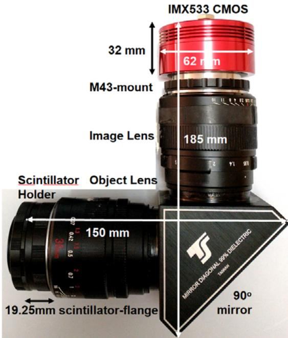
The Compact IMX533 1:1 Macro camera (left) is much brighter than our normal macro camera, with efficiency similar to that of fibre-optic coupling, [according to PCO](#). However the FOV is only ~11x11mm (below left), so we use the smaller [IMX533 square CMOS detector](#) (uncooled for short exposures). The face-to face 35mm f/0.95 lenses are focussed to infinity to give a 1:1 macro image of our 50 $\mu$  wire grid with 3.76  $\mu$ m pixels (below right).
