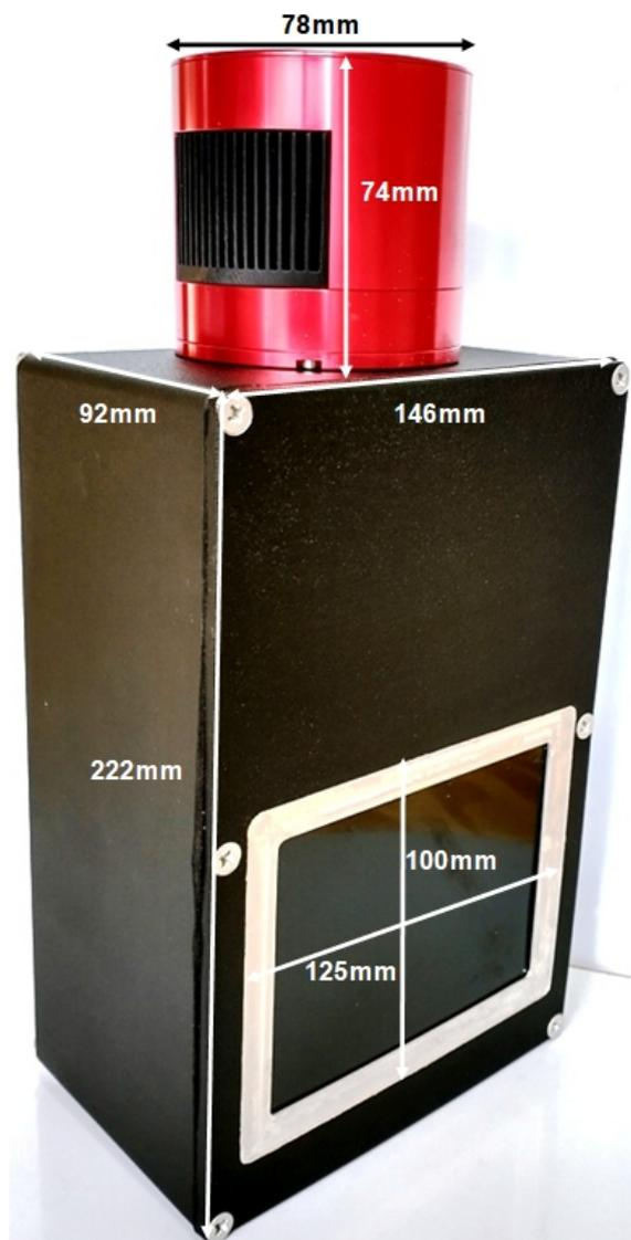
The camera is shown at left with a black-coated CAWO Agfa-Gevaert OG2 x-ray scintillator, but neutron scintillators behind thin aluminium windows can also be supplied.
