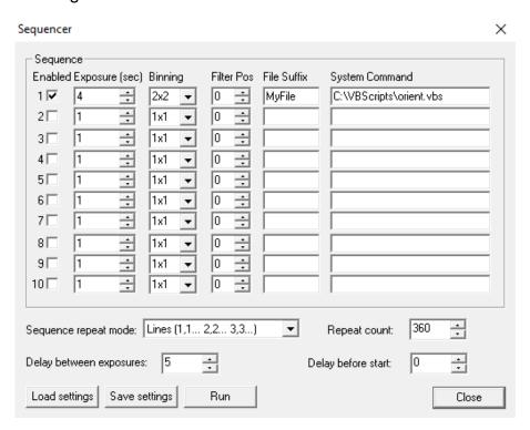
**For Laue diffraction** binning of 4x4 can be used to increase efficiency by a factor of x16! Try also the Infinity software, which allows you to see the image as it is built up by stacking shorter exposures.
